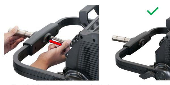
3. Thread the junior pin bolt in through the under side of the mounting yoke, making sure that the bolt engages the threaded hole in the junior pin. Tighten securely with a 10mm hex key. The junior pin is now ready for attachment to a clamp or stand.
